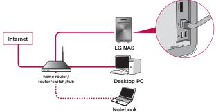
B. If the LG NAS is connected directly to the PC without another network device, it must be connected directly to the PC using a LAN cable, and then the IP address must be set to 192.168.1.201 and the subnet mask to 255.255.255.0.
